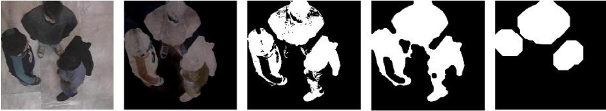
Figure 7 Object detection output for a car with three passengers
