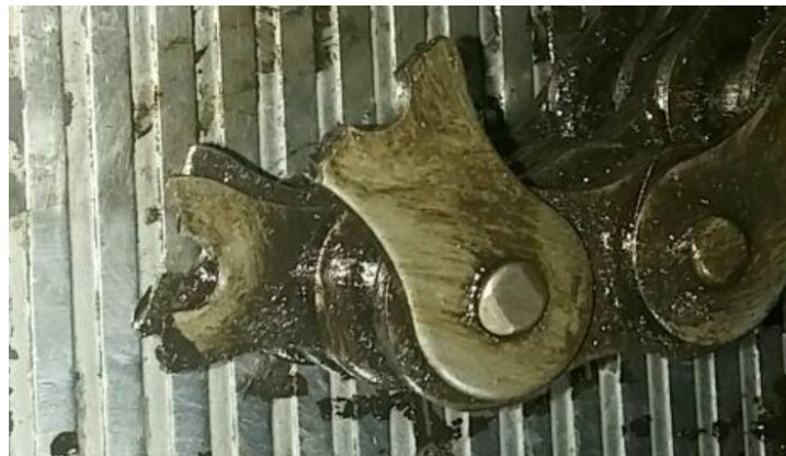
Figure 4 Main chain breakage
