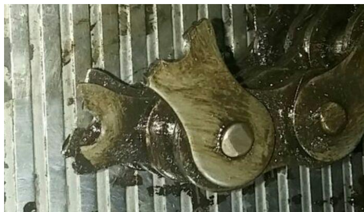
Figure 4 Main chain breakage
