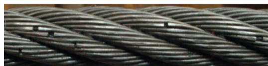
Figure 7 Fatigue-Induced Wire Breaks in Steel Wire Ropes.
