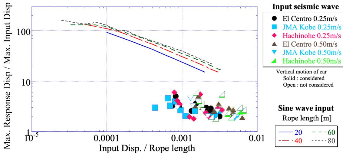
Figure 6 Maximum response displacement of seismic response
