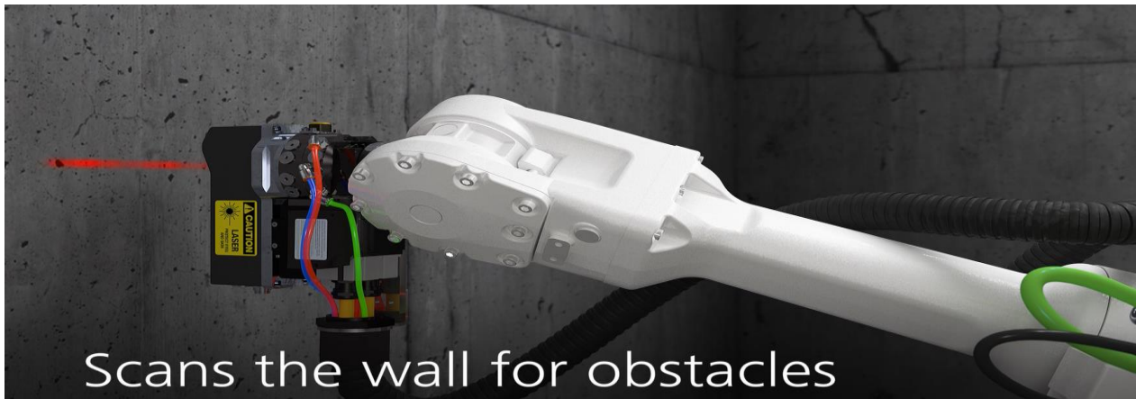
Figure 7 Wall surface scanning and obstacle avoidance.
