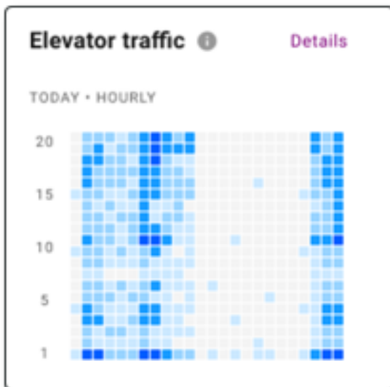
Figure 14 Heatmap of the utilisation of a 20-storey lift over a 24-hour period
