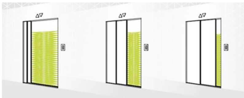
Figure 1 Image of a light curtain during an automatic door closing sequence
