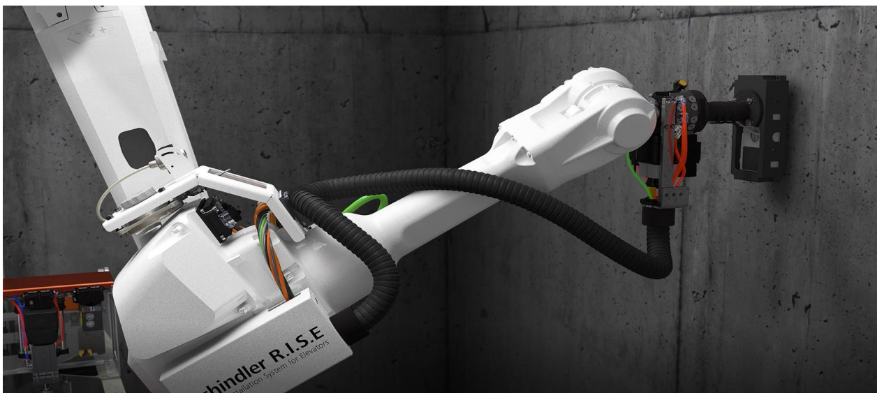
Figure 8 Drilling position calculation based on rebar/wall scan.
