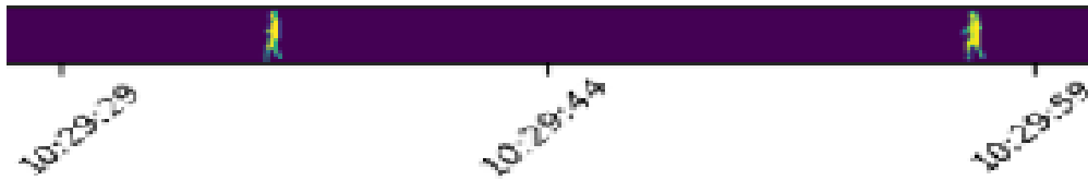
(a) Scanned image of one person entering and exiting a lift over time
