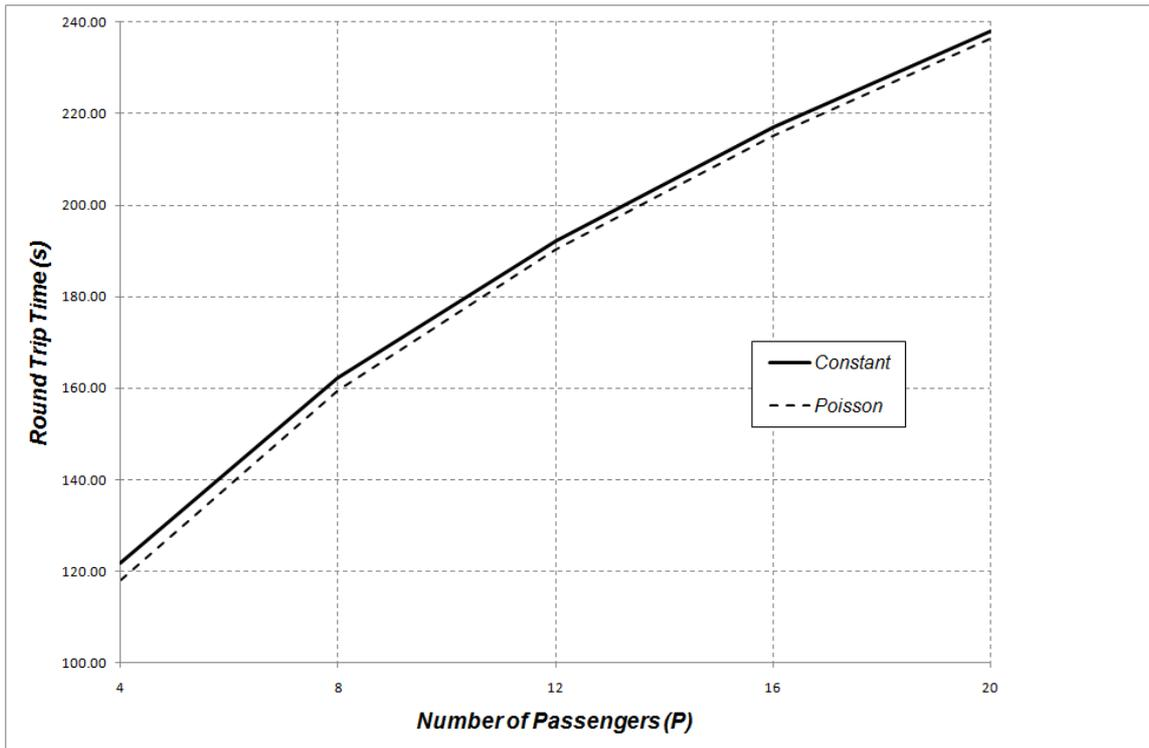
Figure 1: Round Trip Time for a 16 floor building for both constant and Poisson arrival passenger models.
