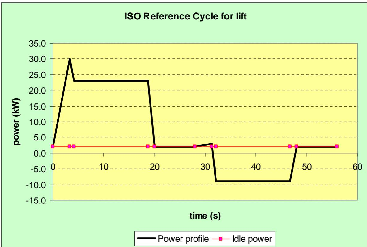
Figure 3 Model plot for installation of Figure 2 (1800 kg lift)
