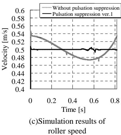
Fig.3 Pulsation suppression mechanism ver.1
