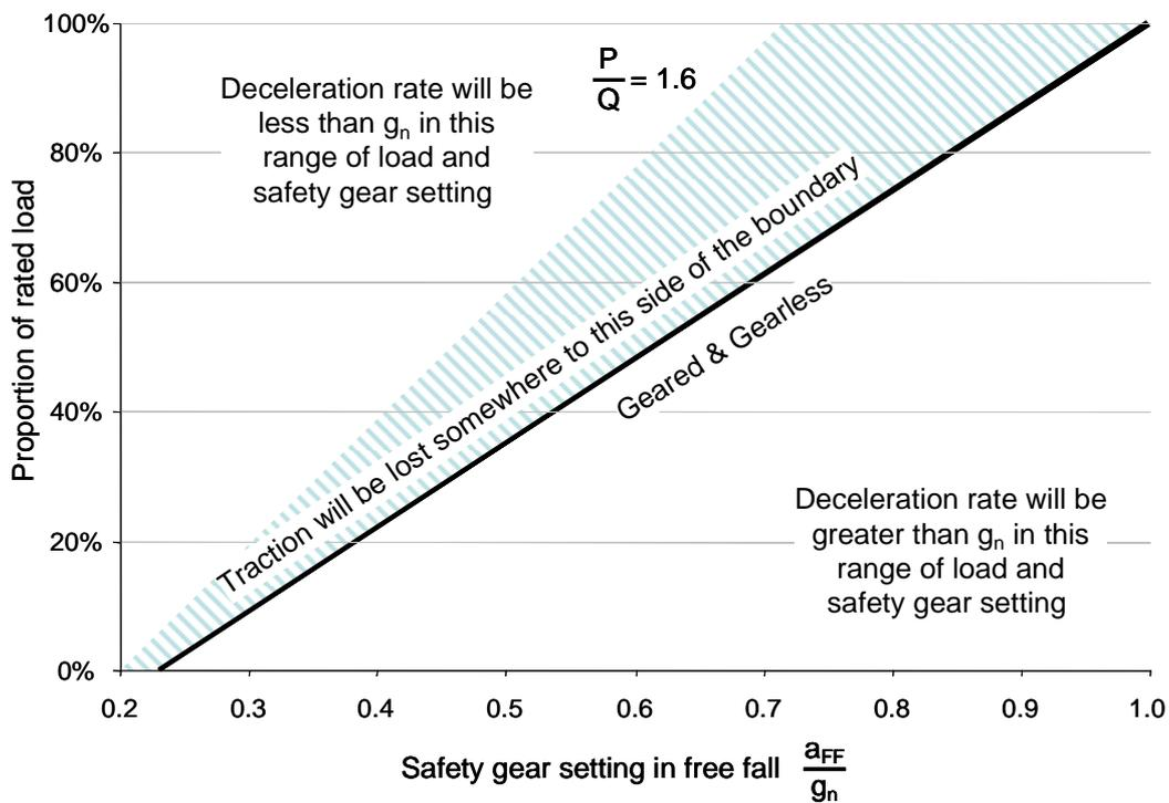
**Figure 2 : Safety gear performance in free descent**
