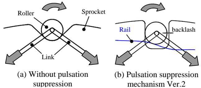
Fig.6 The cause of generating of speed pulsation
