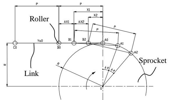
Fig.1 Pattern diagram of an escalator drive part
