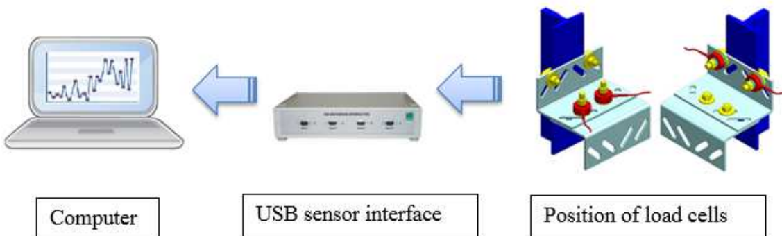
Figure 5: Data acquisition and signal processing [2]
