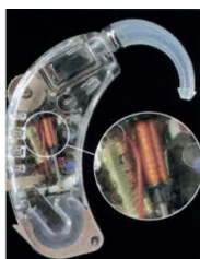
Figure 1 'Telecoil' in hearing aid
