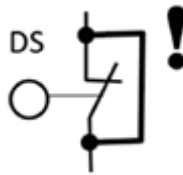
Figure 4: Bridging switch sign [Source: DIN EN 81-20]
