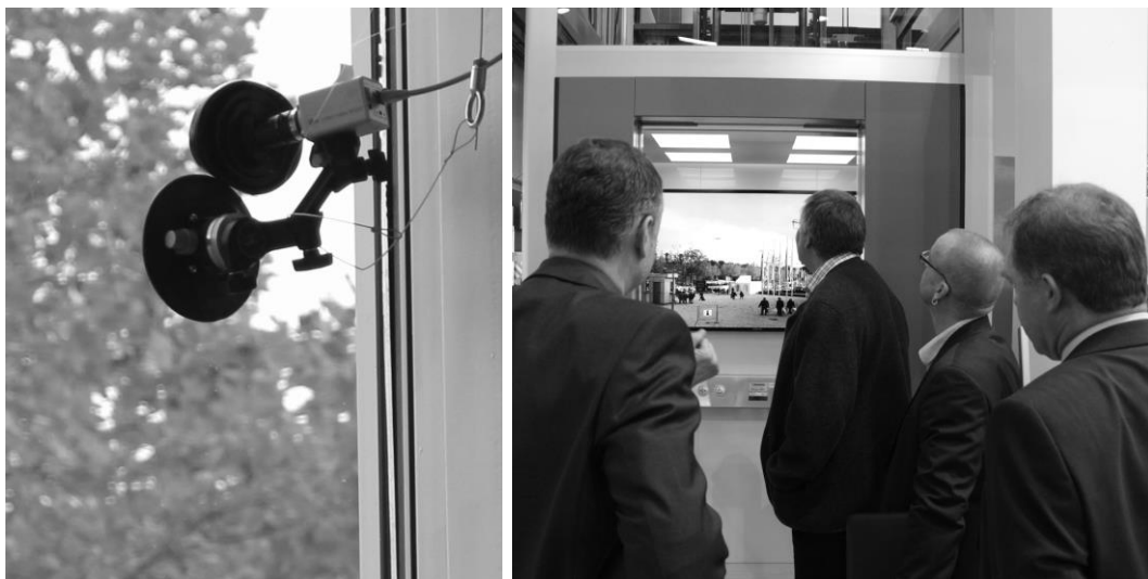
Figure 5. Case of live, real time virtual window: one of two HD cameras mounted on building façade (left) and HD LED display mounted on rear wall of lift (right). Augsburg, 2013
