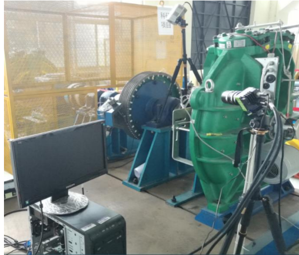
Figure 3 Structure of slippage measuring equipment
