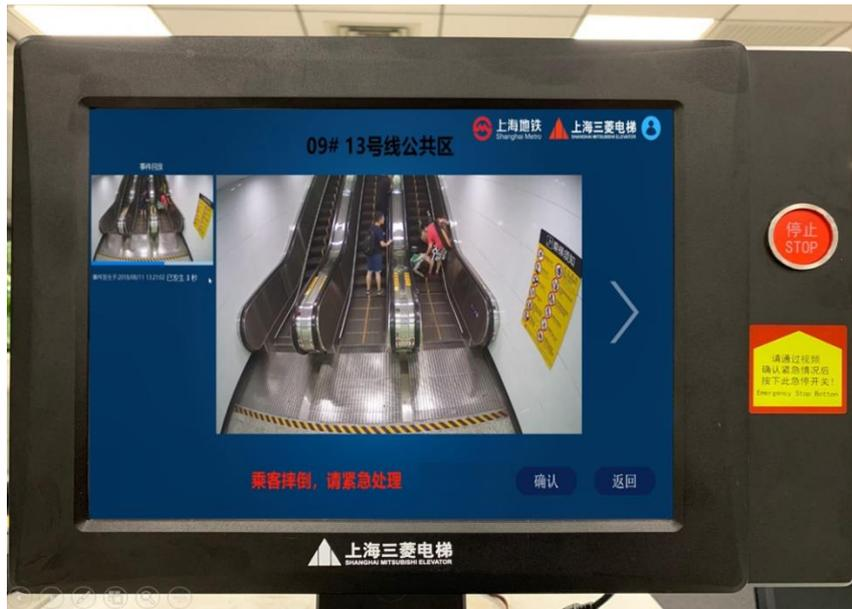
**Figure 4. Monitor screen and the actual stop button**
