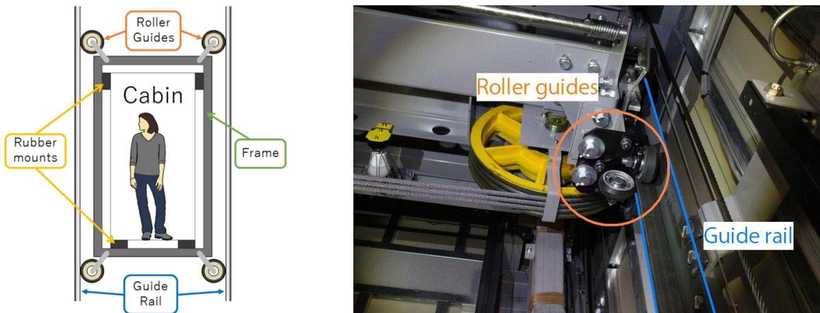
Figure 1 Structure of lift cabin
