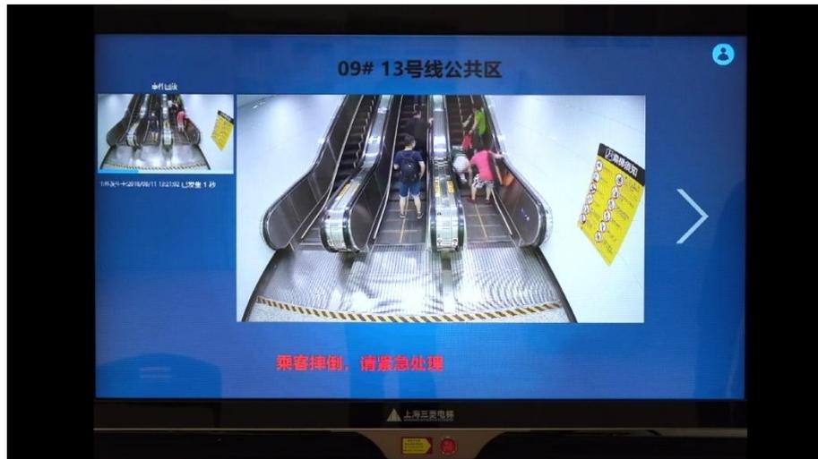
**Figure 5 Passenger fall detection and remote stop of escalator**
