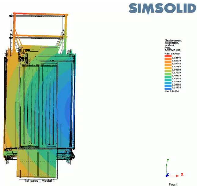
Figure 6 Eigenfrequency extraction for sling-car-doors subsystem with meshless method
