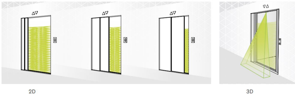
Figure 4 2D light curtain combined with a 3D ToF sensor
