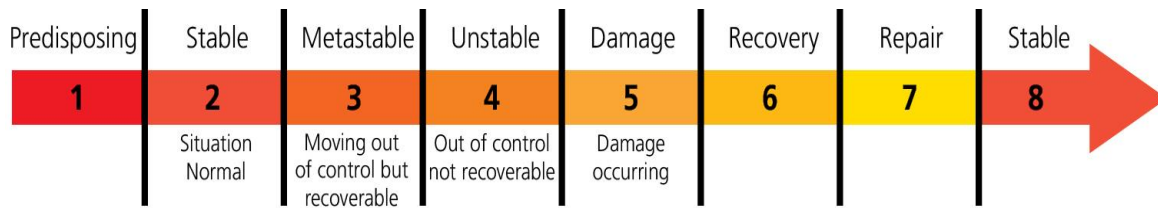
Figure 7 Unscaled time diagram for an incident resulting in death or destruction of equipment. Incidents with less serious outcomes branch from this time diagram at any stage [11]
