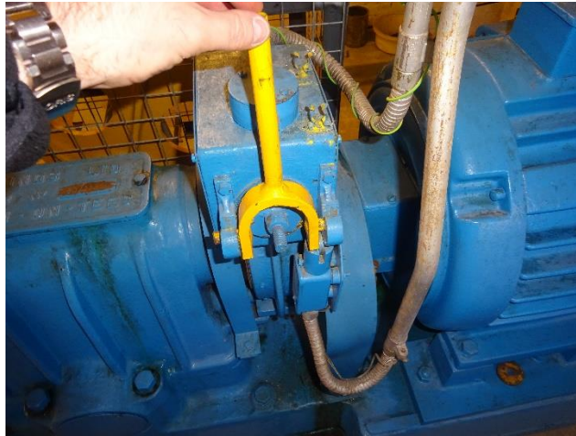
Photograph 1 Example of a brake release that can permanently jam open
