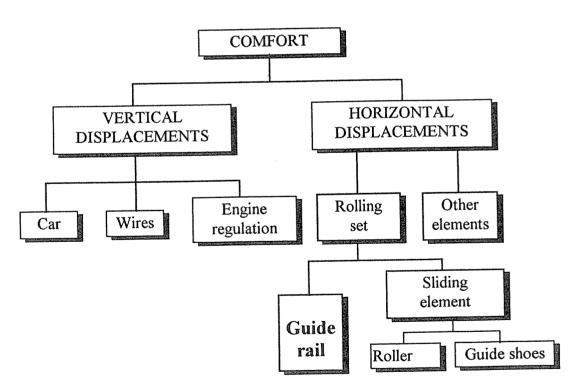
The Guide rail, apart from being a basic element for the elevator safety, is the element with greatest incidence in the COMFORT as it is the way the elevator slides along. Any irregularity, either in the manufacture or in the assembling can be appreciated by the user.
