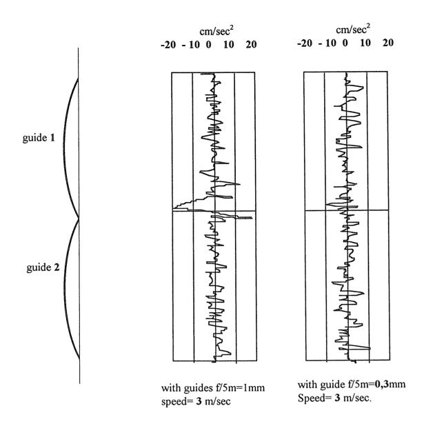
We have also verified that as speed increases, the accelerations are bigger because of 5m/deflection. Nevertheless, COMFORT is not influenced significantly. Where problems are originated is at the joints when assembling guide rails with the bending in the same sense.
