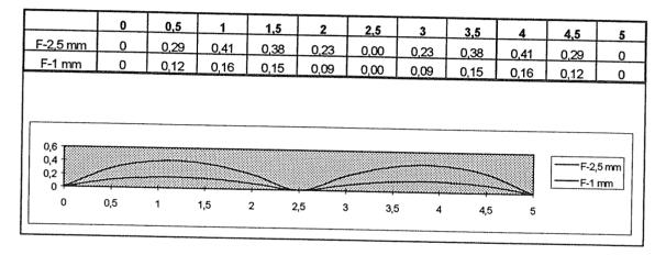
As it can be seen in the graphic, when forcing the guide rail in the middle so as to straighten it, what we are doing is to create 2 curves that, although with lower values, can have negative influence.
