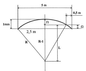
A guide rail with a uniform bending of 1mm maximum deflection (extraquality guide rail) is considered here.
