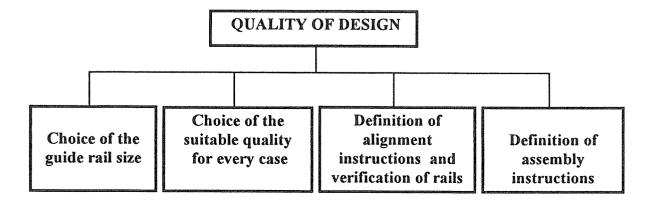
Choice of the guide rail size.- It is usually done taking as a basis only the calculation of efforts produced in both the elevator displacement and the safety gears performance, without comfort being taken into consideration. The side accelerations produced in the elevator depend on its features:
