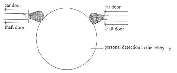
A little better are sensitive edges in front of a moving mechanical edge, because the reacting zone is wider; and they have electrical switches to stop the door, if the mechanical edge is moved.
