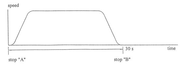
2. Measurement of running time from level "A" to level "B" with one intermediate stop
