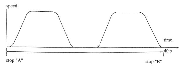
3. Measurement of door holding time during one intermediate stop. The door holding time in this example is measured with 4 s.
