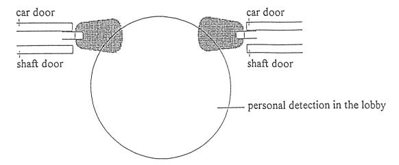
At the moment I think the light screens to be the better solution. There are also light screens which do not react to objects in the complete area between the door edges but only to objects which are in a reaction zone of nearly 200 mm in front of the door edge. For every system, the braking distance of the door has to be smaller than the reaction zone of the door edge monitoring system.
