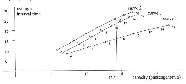
All curves in both diagrams show elevators in a building with 12 floors above the main terminal, a floor height of 3.50 m, and a population of 40 people on each floor. If the desired 5 minute peak rate should be 15 %, the required handling capacity for this building is 14.4 passengers per minute. A 15 % 5 minute peak rate is good for a comfortable office building with one or two tenants.
