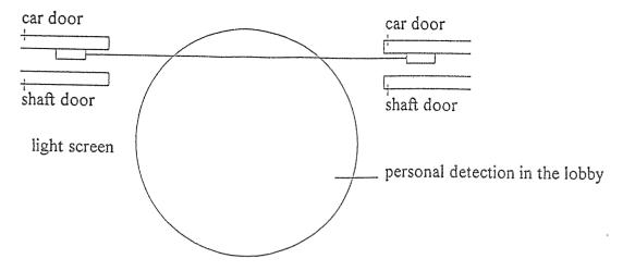
Sensitive edges have an electrical field and react to objects which interrupt the field lines. They detect the complete space in front of the door edges. But they do not function independently from differing weather conditions and their function is very dependent on the quality of the maintenance and service personal.
