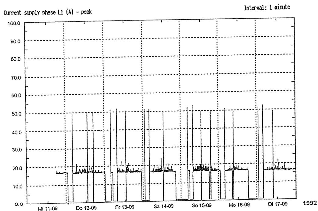
From the form of current curve it can be deduced that the power factor is about  $\cos \varphi = 0,85$ . Three starts average per day have been registered.
