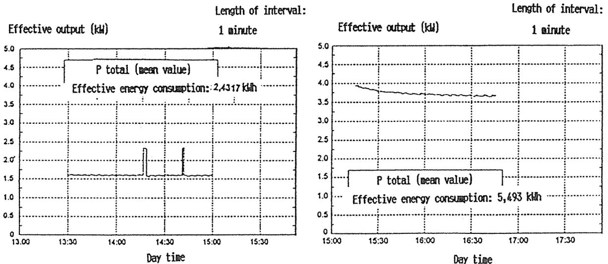
The saving through the reduction of true energy consumption extrapolated over a period of 12 months can be best seen from the next graph. Over 6000 KWh per year can thus easily be saved.
