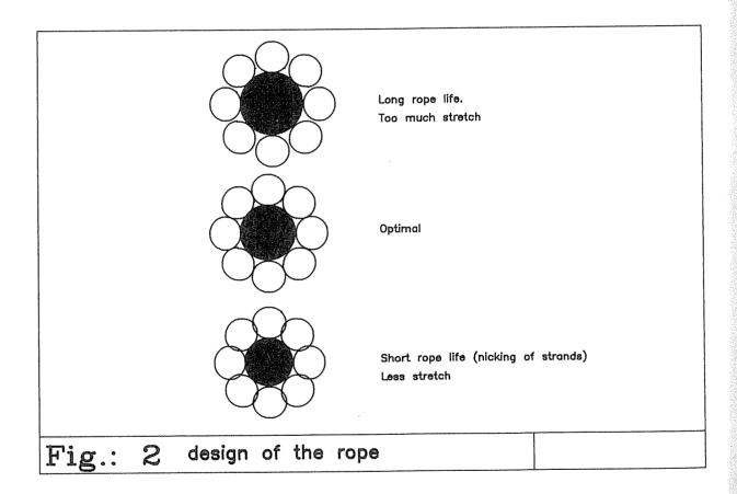
From the next 3 rope cross sections (fig. 2) it will be clear that number 1 has a long fatigue life with the most stretch. More often shortening of the rope will be the result. Number 3 will have less stretch but the rope life will be short due to nicking of the strands with many wire breaks. At the end the strand will break.
