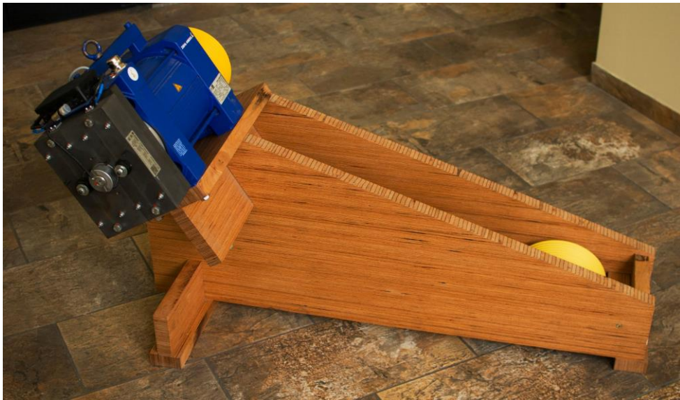
Figure 7: Machine frame made entirely of wood
