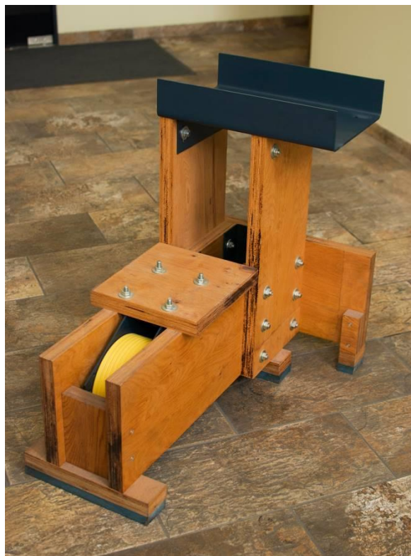
Figure 8: Machine frame made primarily of wood
