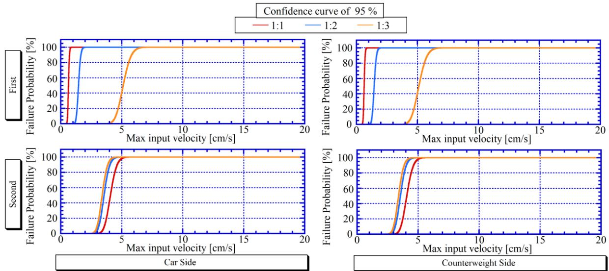
Figure 12: Fragility curve of model B of compensation rope
