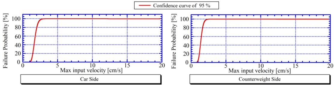
**Figure 9: Fragility curve of model A of main rope**
