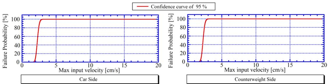
**Figure 10: Fragility curve of model A of compensation rope**
