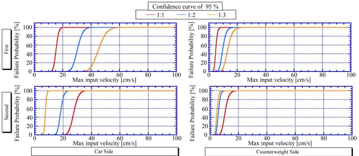
**Figure 11: Fragility curve of model B of main rope**
