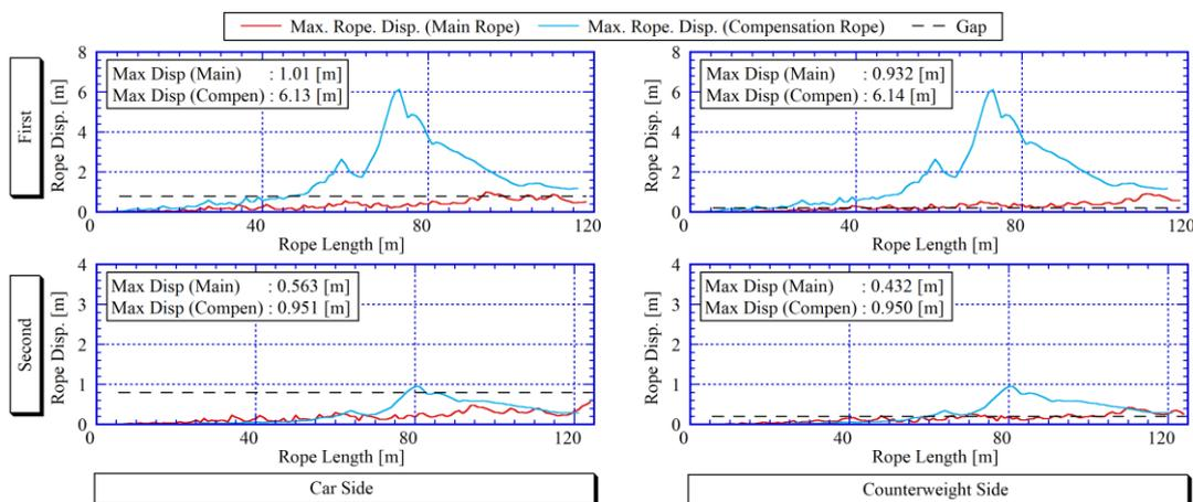
Figure 6: Numerical result of model B (1:1)
