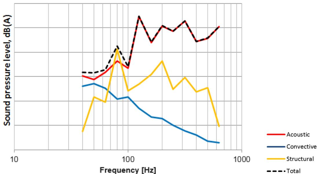
**Figure 7 Influence of different sources on in-car noise**
