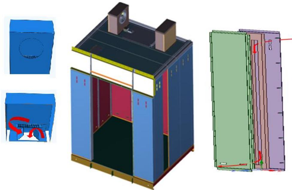
**Figure 4 Car structure and details: fans, car, panel structure**
