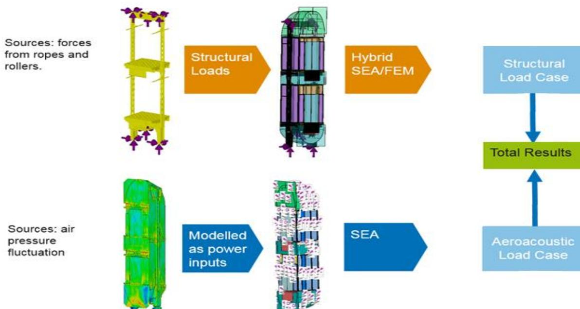
Figure 1 Noise sources in the lift car
