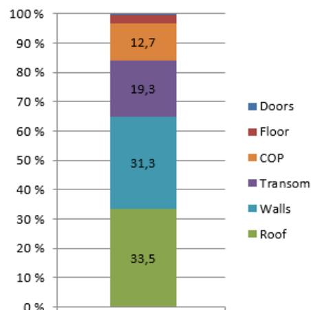
**Figure 9 Ranking the noise sources based on components**
