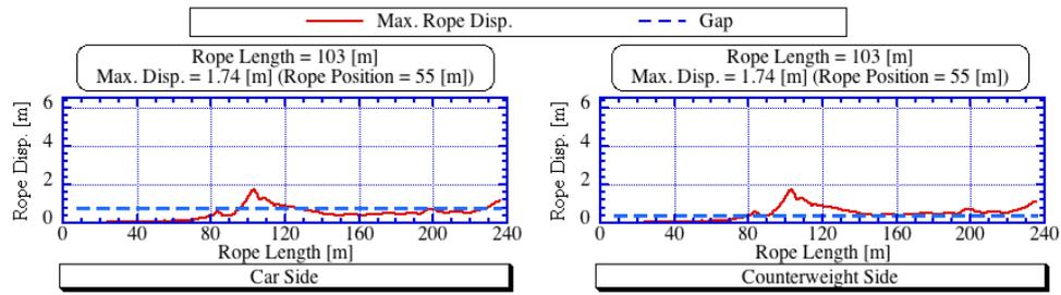
**Figure 8. Numerical result of model A of compensation rope**
