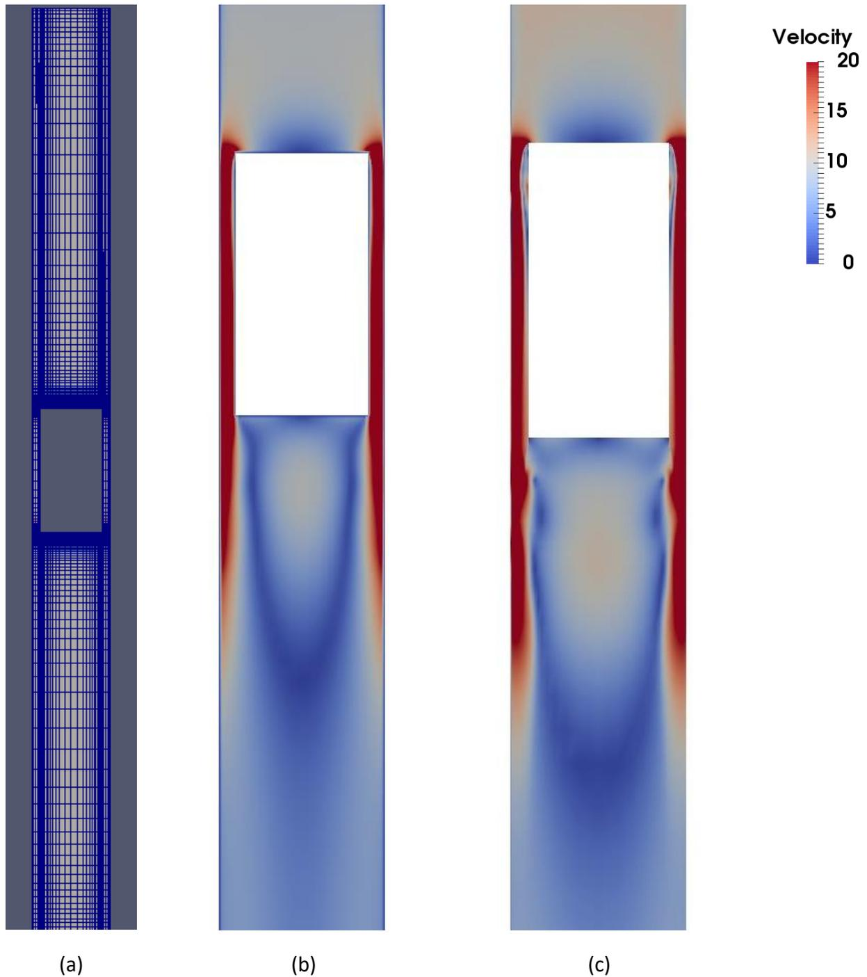
**Figure 1.** (a) CFD mesh. (b) Velocity contour (RANS). (c) Velocity contour (DES with  $K-\omega$  SST).
