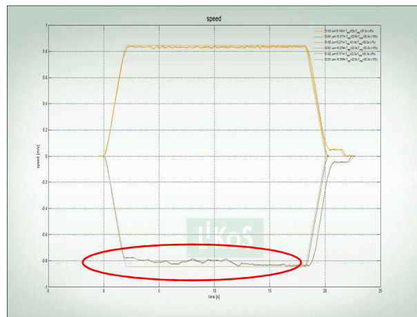
Figure 2 Speed curve of lift
