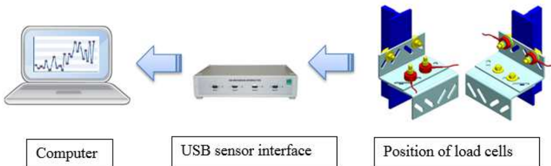
Figure 5: Data acquisition and signal processing [2]
