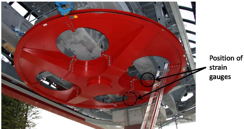
Figure 9 Sheave of a rope way
