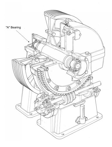
The forensic analysis also showed high levels of 'wear metal' elements (Copper -Cu and Tin -Sn) in both samples – these 'wear metals' originated from the sliding friction between the phosphor bronze
