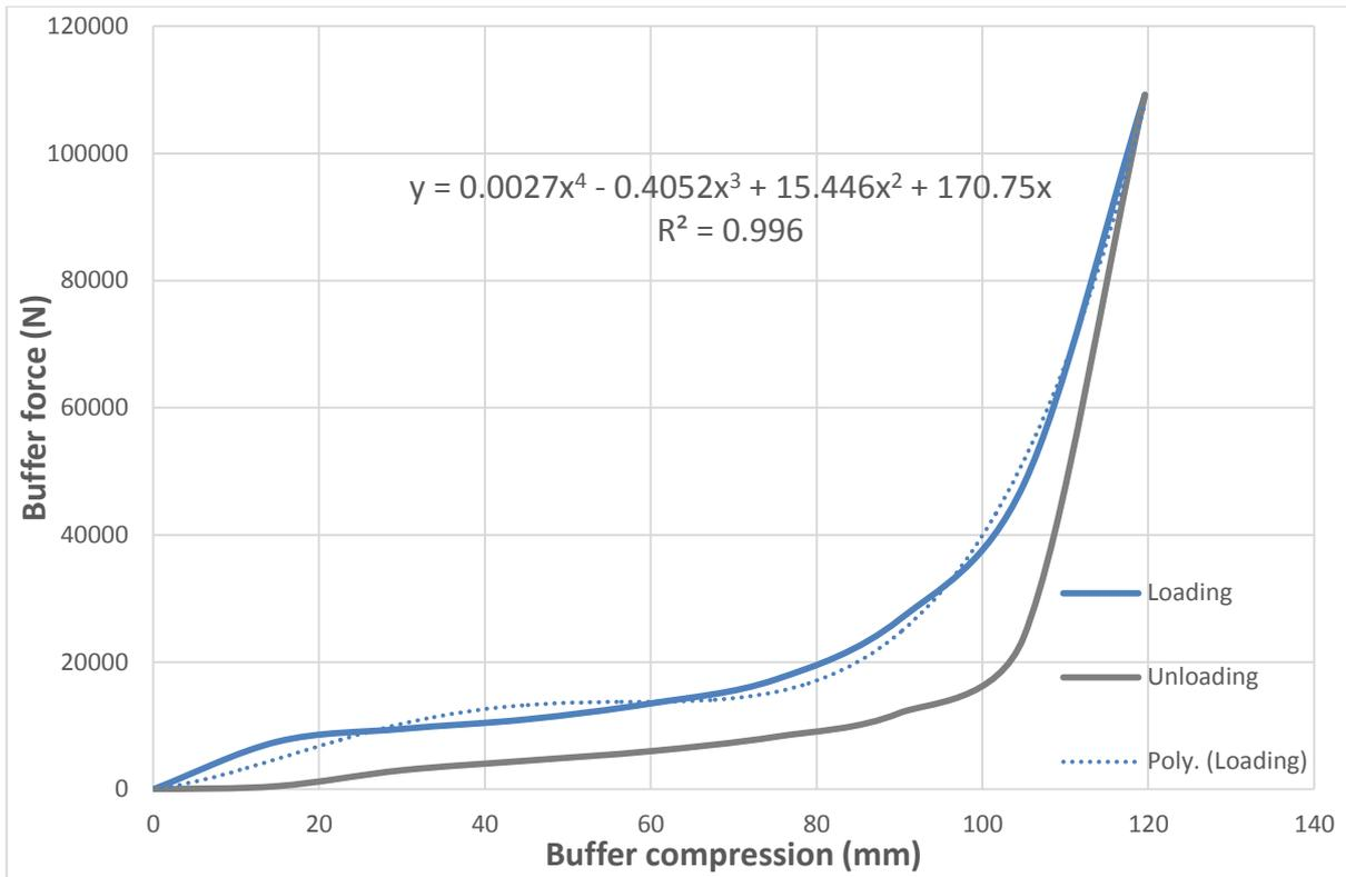
**Figure 2 – Typical non-linear buffer characteristic curve**
