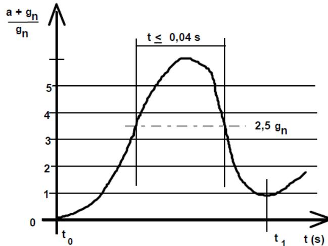
$t_0$  = moment of hitting the buffer (first absolute minimum);
