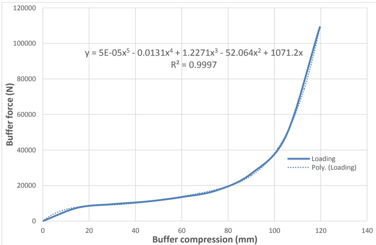
**Figure 3: Typical characteristic curve and 5<sup>th</sup> order polynomial fit**
