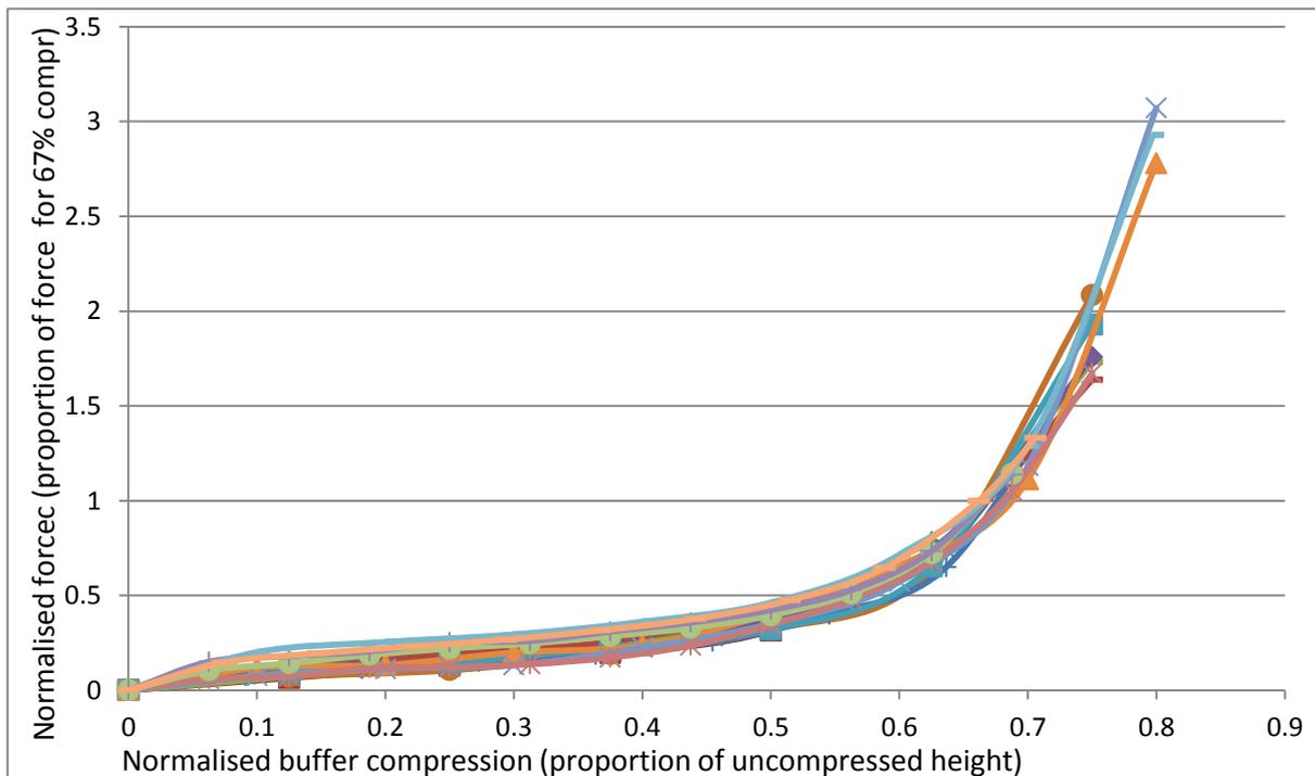
**Figure 4: normalised buffer characteristic curves for 18 buffers studied**
